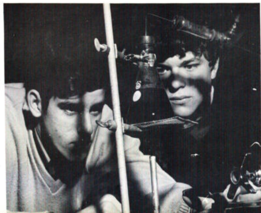
To isolate ethyl alcohol from a complex mixture, Tom Beneventi and Bob McDowell use a fractional distillation apparatus.
