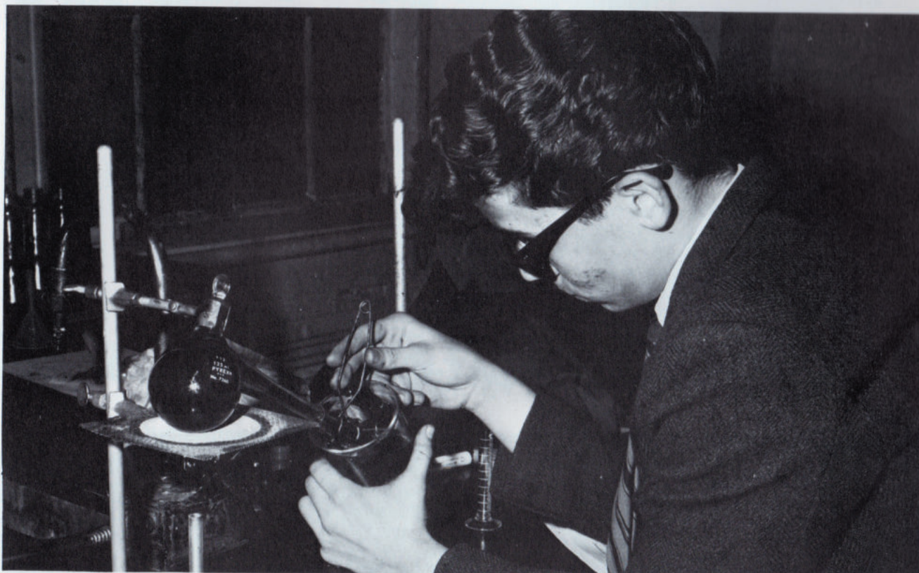
Combine potassium bromide, manganese dioxide and sulfuric acid in a retort; heat gently. Collect the vapor given off in a
