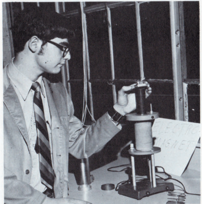
Using different metal rings and an electromagnet, Siro Pieri demonstrates the parameters effecting Lens' law.
