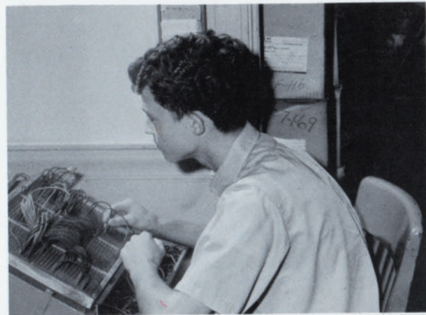
The preparation of a program for the accounting machine is wired on a control panel by Senior Jim Wilson.
